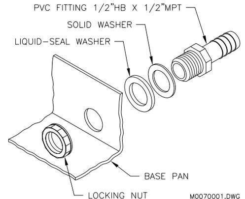
For installation of the condensate drain:
